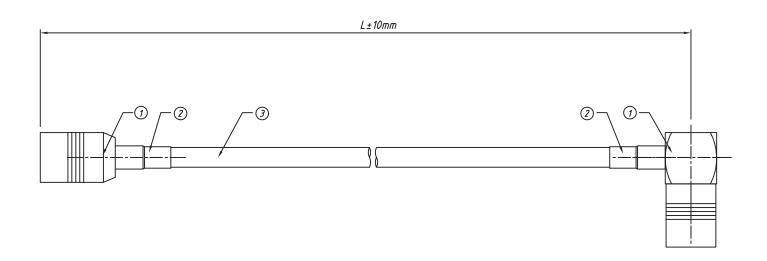
SMB plug,Female to SMB plug,Female R/A Cable
